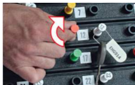
The user access peg is inserted to remove the desired key from the system
